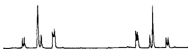
Figure 5. Fluorine, 19 F, -{ 19 F r } nuclear magnetic resonance spectrum at 56.4 Mc.p.s. of perfluoro-1,2-dimethylenecyclobutane: (a) observed, (b) calculated.
